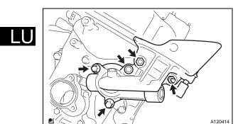
3. INSTALL OIL FILTER BRACKET SUB-ASSEMBLY
