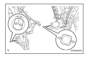
(e) Align the key way of the oil pump drive rotor with the rectangular portion of the crankshaft timing gear, and slide the timing chain cover into place.
