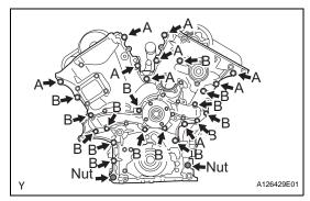
(f) Install the timing chain cover with the 24 bolts and 2 nuts. Tighten the bolts and nuts uniformly in several steps.
