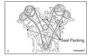
(d) Apply continuous beads of seal packing (diameter 3 to 4 mm (0.12 to 0.16 in.)) to the timing chain cover as shown in the illustration.
